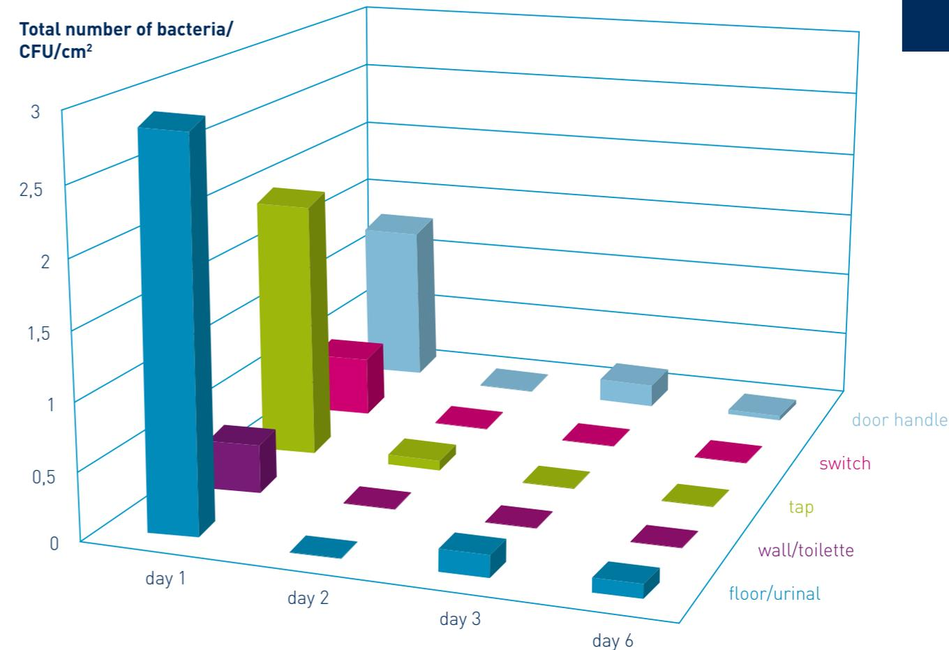
The long-term effectiveness of the CleanO<sub>3</sub> mat has been confirmed in a field test under real conditions: Before the first disinfection cycle the numbers of bacteria were measured at various locations in a toilet. This showed comparably high levels. The 35-minute disinfection cycle then always started whenever the user of the toilet
