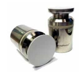
The X2534 ValProbe surface temperature logger design provides enhanced and precision wireless measurement capability ideal for freeze dryer shelf temperature measurement over an extended temperature range from -85°C to +140°C.
