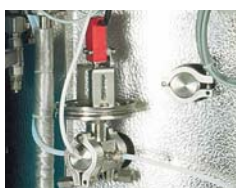
FVG - Membrane safety device for preventing lid opening even in case of minimal over pressure
