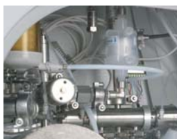
Diaphragm valve in AISI 316 L stainless steel with pneumatic actuator & decontamination of exhaust air with sterile filter
