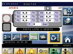
DCS PLUS 10 process controller
